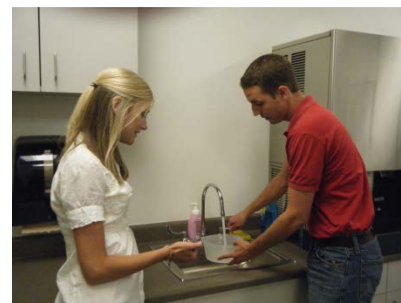
Measuring the rate of flow from a faucet
