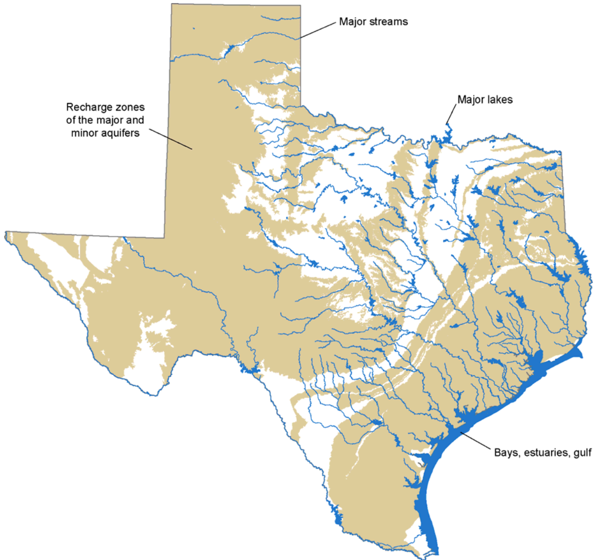
Figure 2: Areas in Texas where streams overlie the recharge zones of the state’s major and minor aquifers.
